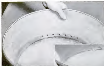
The drain holes are at the bottom. From them, the water flows into a drainage apron and out through the overflow spout at top
